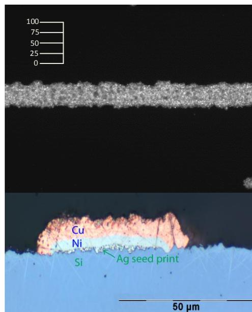
**Figure 2:** Top: Image of inkjet seed & Cu plate finger of the front grid. Bottom: cross section. Seed print Ag mass was in this case 2.4mg for the grid fingers.
