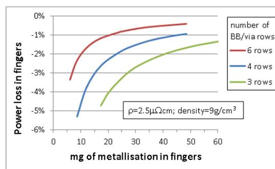
**Figure 1:** Illustration of the benefit of multiple contact rows (i.e., busbars, or vias in the case of MWT cells) for paste reduction potentiality. Figures apply to one cell side.
