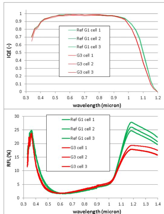
**Figure 4:** Internal quantum efficiency and front escape reflectance of n-type cells with Ag fire-through grid and n-type cells with Al-PVD rear metallisation
