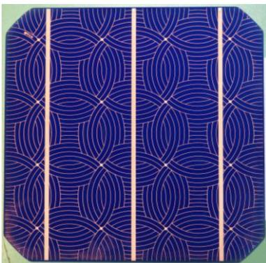
**Figure 3:** Photograph of Cu-plated n-type MWT cell with 16 vias. The three busbars would normally not be present in the MWT grid, but were in this case added as an improvised means to connect to the electrical contacts for the plating.
