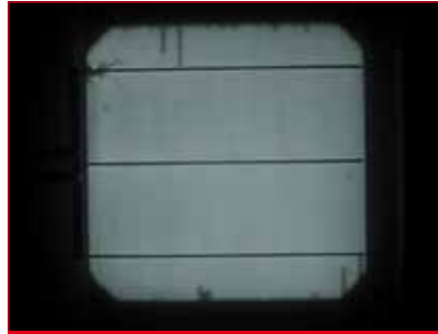
Figure 8. EL image of an H-pattern single-cell module with soldered front-side contact and MWT rear-side contact, showing cracking in the top left corner and finger interruptions at the edges of the cell.
