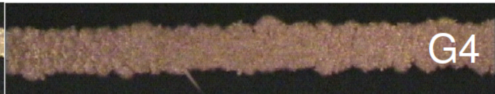
After NiCu plating (2+8 \mu\text{m} ): width 55-60 \mu\text{m}
