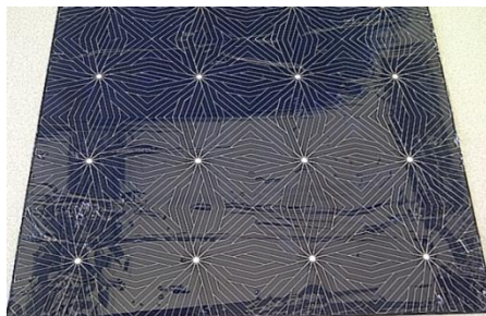
undamaged solar cell (clean by incineration)
