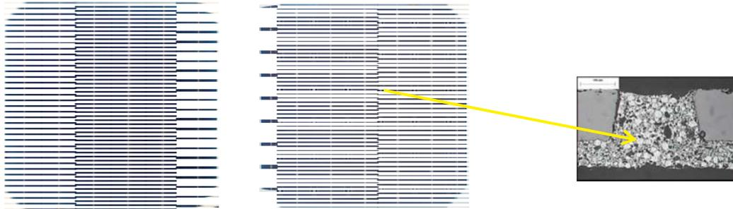
Figure 1: front and back of a high efficiency bifacial metal-wrap-through cell, with cross section of wrap through metal contact
