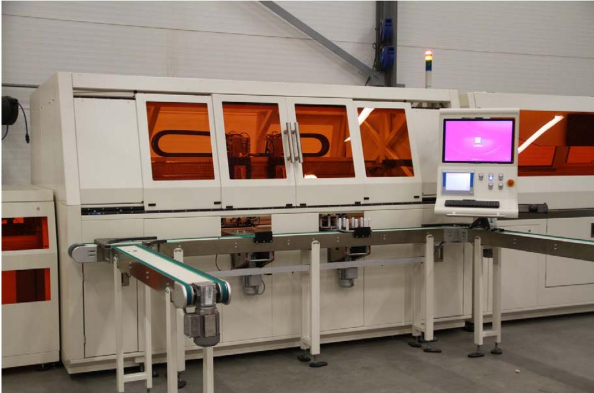
Figure 18: Picture of the new developed Cell Positioning Unit, particularly suitable for IBC cells and other cells which require extra accurate placement.
