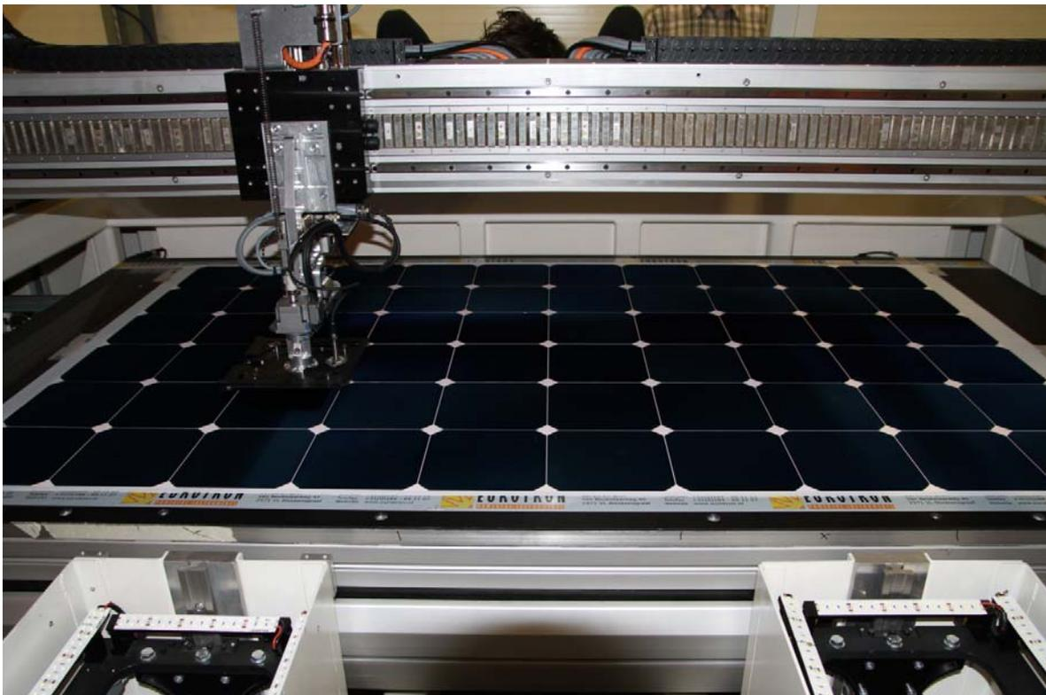
Figure 19: The full size module containing all aspects of the Cu-PV technologies in the pick-and-place cell placement machine.
