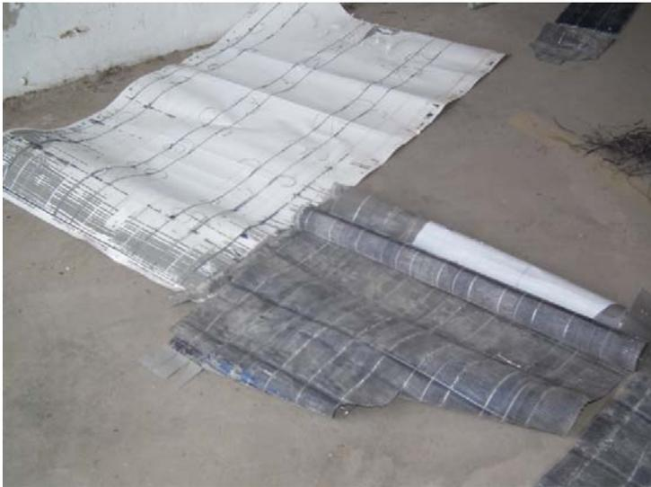
Figure 22: Back sheet (left) and EVA-silicon cell sandwich (right)
