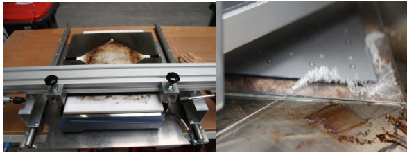
Figure 3: Photo of the wire saw set-up used to separate the solar cell from the glass by cutting through the thermoplastics-based encapsulant
