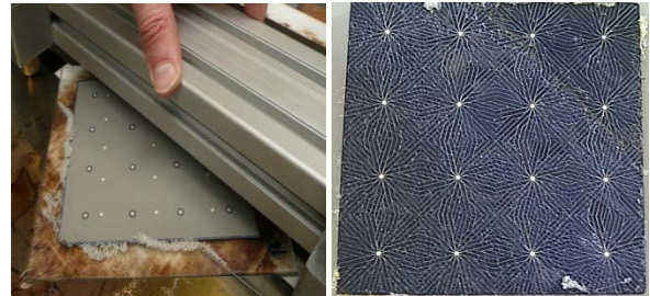
Figure 8: Separating solar cell from glass sheet for thermoplastic-based module. The separated cell is shown on the right
