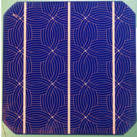
Figure 4. Photograph of Cu-plated n-type MWT cell with 16 vias. The three busbars would normally not be present in the MWT grid, but were in this case added as an improvised means to connect to the electrical contacts for the plating.
